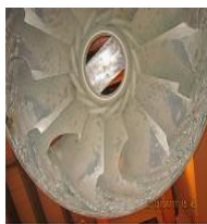
48MW Francis Turbine at Kaligandaki Power Plant, Nepal[24]
